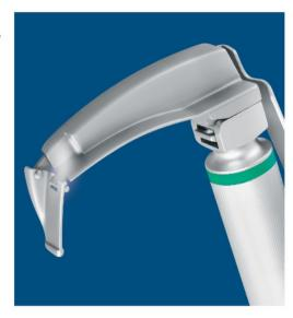
Sun-Flex is a modified English Profile Macintosh laryngoscope blade with a tip which is adjustable. A lever controls the tip angle during intubation to lift the epiglottis, giving a clear view of the vocal cords. Contact with the upper row of teeth and unnecessary pressure on the tongue and soft tissue are avoided.
